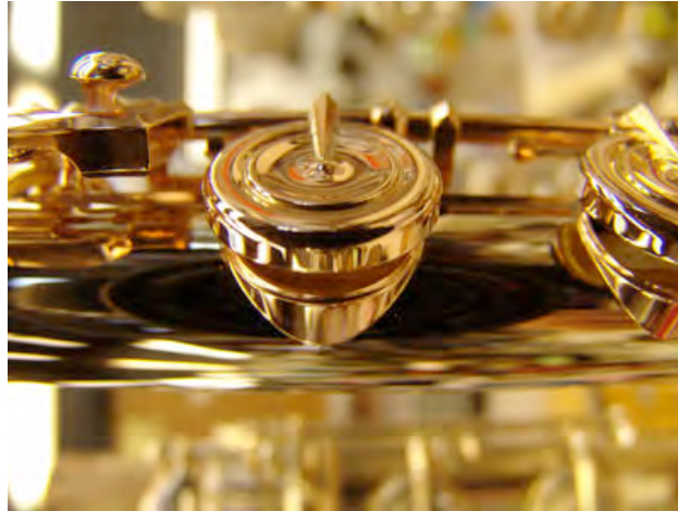
An Example of Pointed French Arm Keys
